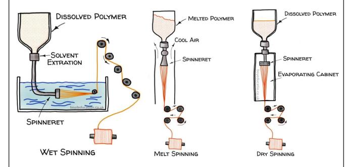
All 3 methods extrude a polymer solution through a spinneret. Explain what this means.
